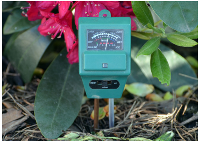
A soil moisture sensor in soil
